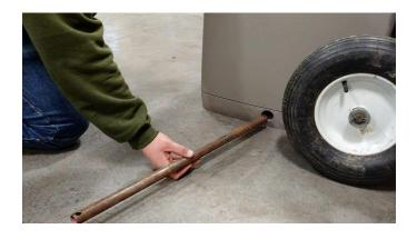
Insert second crossbar into back of generator shipping holes. This crossbar should have only two holes on top to allow straps to be connected.
