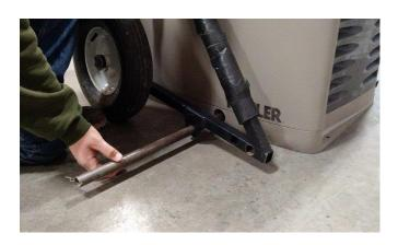
Insert crossbar into front generator shipping holes. Install cotter pins to secure bar.
