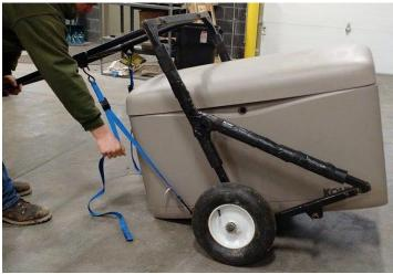
Push down on handle and pull down on blue harness straps. The lower you push the handle down while pulling down on the blue strap, the higher the generator clearance off the ground.
