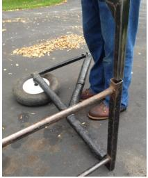
Slide the left and right wheel assembly into the handle assembly. Slide the assemblies all the way into the handle. Tighten knobs for a rigid connection.
